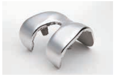
電子ビーム積層造形で製造したCo-Cr-Mo合金製人工膝関節 Artificial knee joint made of CoCr-Mo alloy fabricated by EBAM.
