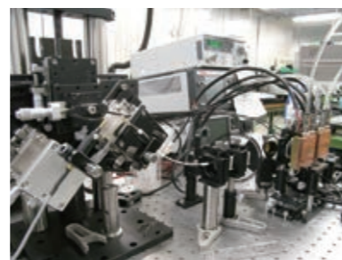
赤外光を用いた血糖測定器 Blood glucose measurement system using infrared light
