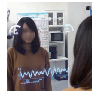
鏡型生体信号計測デバイス Mirror type device for non-contact measurement of biological signal
